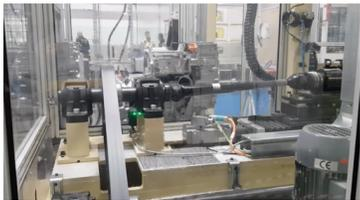
AsystemPredict's wake up on vibration feature is used to collect real time data on the test bench condition
