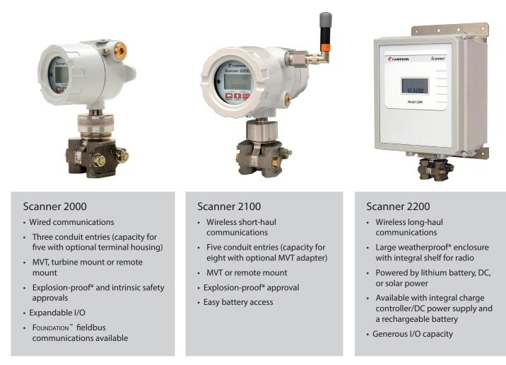
CAMERON Scanner 2000 series flow computers are among the most versatile flow measurement devices on the market. Each device can operate independently as a flow computer, RTU, or process controller, or act as a node in a comprehensive SCADA network.
