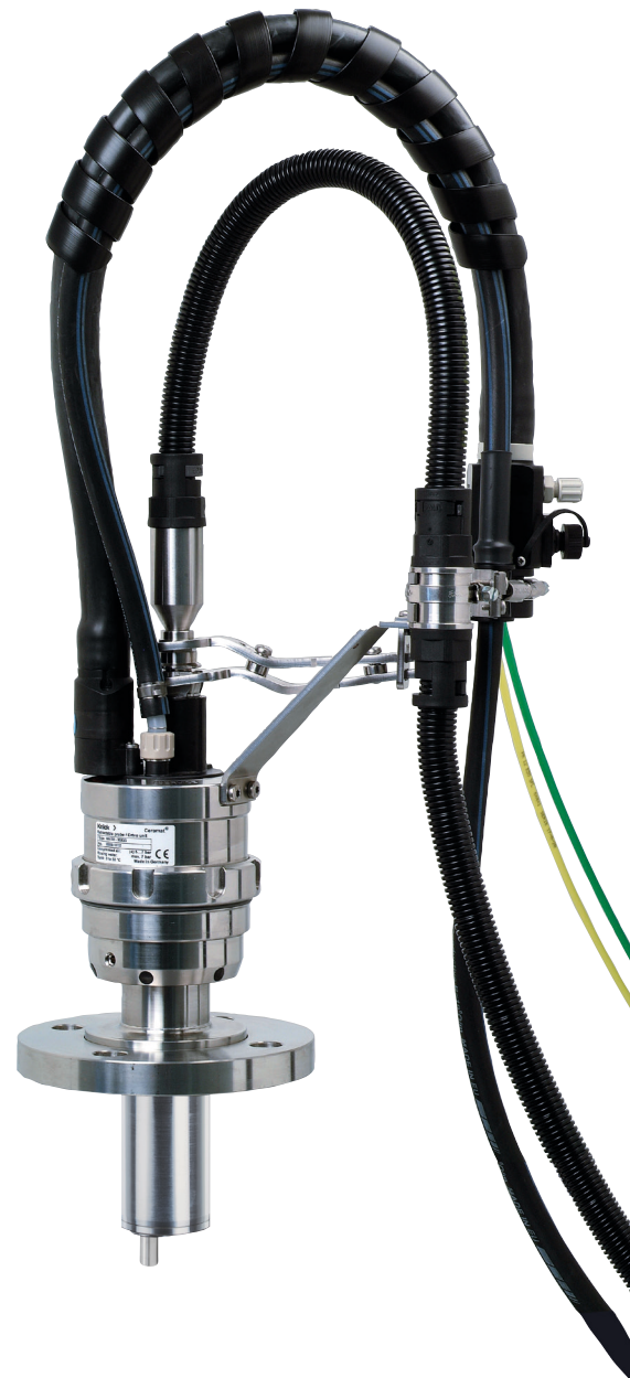
Optical probe Ø 12 mm or Ø 12.7 mm
