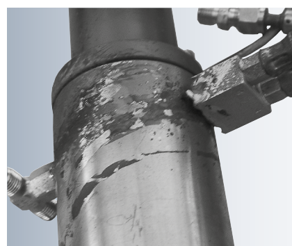
Conventional retractable fittings: Tangled hoses (left) and deposits on unprotected limit-position mechanism (right)
